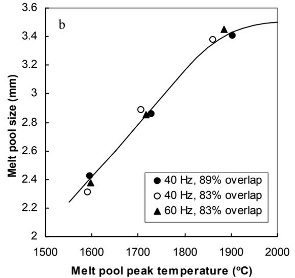
Figure 5. Relationships between (a) pulse peak power and pulse peak temperature and (b) pulse peak temperature and melt pool size.
