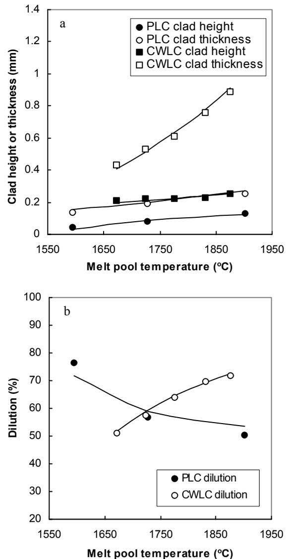
Figure 7. Comparison of (a) clad height and total thickness of clad layer and (b) dilution between pulsed and CW laser cladding on the melt pool temperature.
