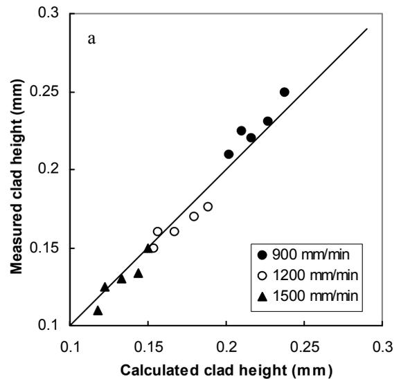
Figure 4. Comparisons between the measured and calculated clad height and total thickness of clad layer for continuous wave laser cladding.
