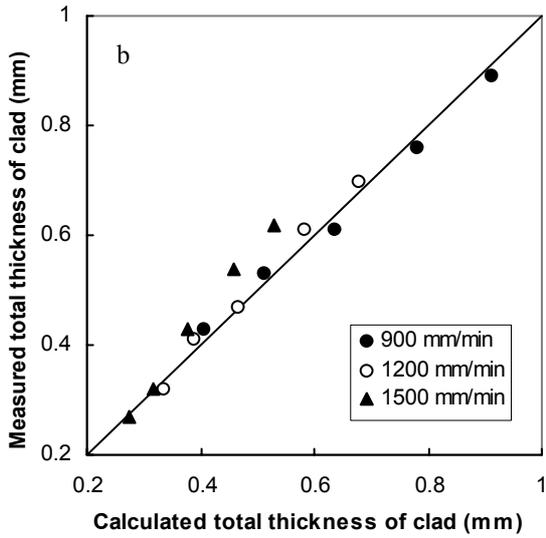
Figure 4. Correlation between the calculated and measured (a) clad height and (b) total thickness of clad layer for CW cladding.
