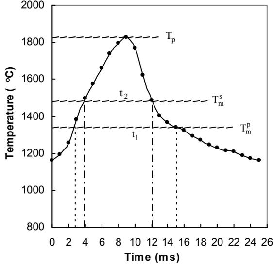
Figure 1. A typical melt pool temperature profile of pulsed laser cladding at pulse frequency of 40Hz. Data points reflect the sampling rate of 1kHz.
