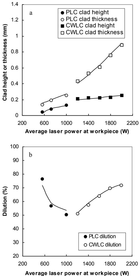
Figure 8. Comparison of (a) clad height and total thickness of clad layer and (b) dilution between pulsed and CW laser cladding as a function of the laser power at workpiece.
