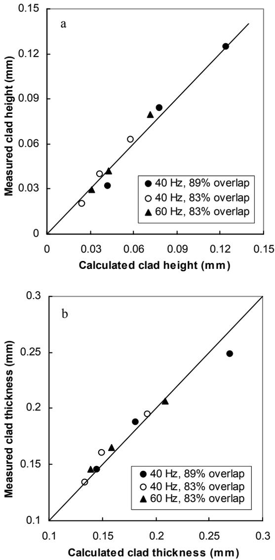
Figure 6. Comparison of the measured and calculated (a) clad height and (b) total thickness of clad layer for the single-track pulsed laser cladding.
