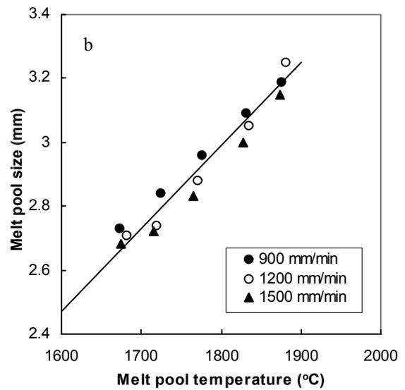
Figure 3. Relationships between (a) laser power and melt pool temperature, (b) melt pool temperature and melt pool size.
