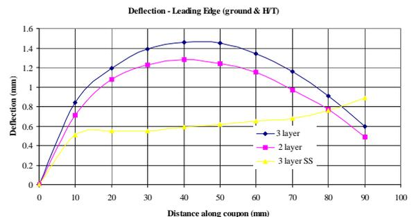
**Fig 6.** Leading edge distortion during cladding.
