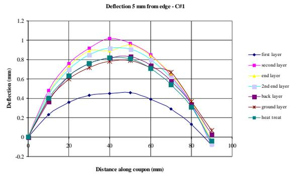
**Fig 5.** Distortion of test coupons during multiple layer cladding of Stellite 6.
