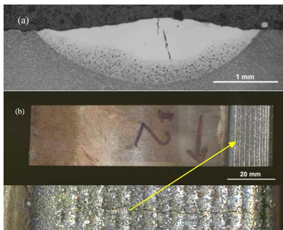
**Fig 7.** Cracking of the Stellite 6 clad (a) within the clad track and (b) across the clad tracks.
