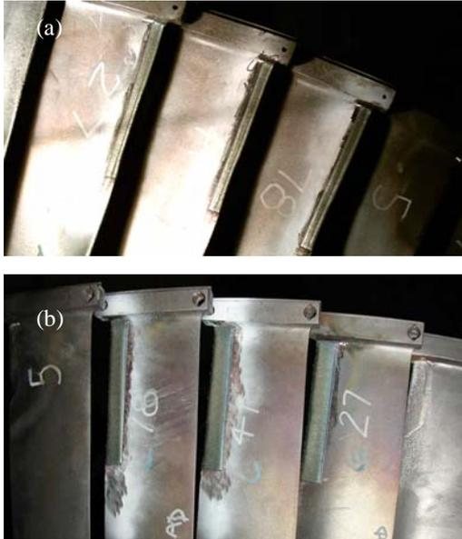
**Fig 4.** Laser clad blades showing (a) front view and (b) rear view before processing to original profile.
