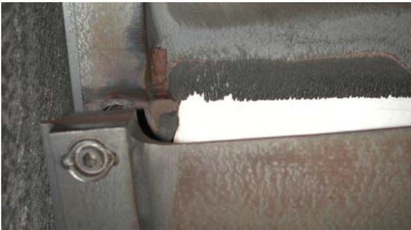
**Fig 2.** Erosion of the blade.
